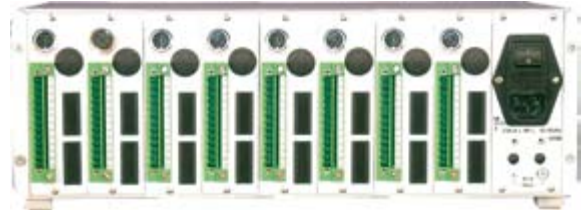
Back view: All sockets for sensors, control signals and serial interfaces are completely installed.
